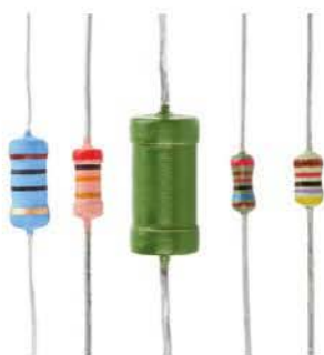
A resistor is a component with a known resistance. You can work out the resistance from the colors.
