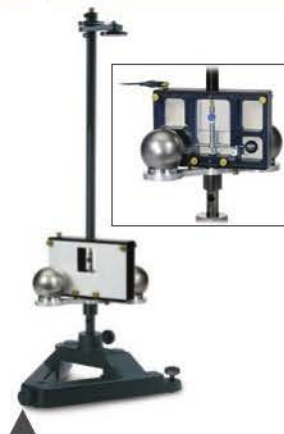
The modern equivalent of the apparatus used by Cavendish to measure G in 1798.
