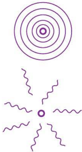
E.2 Figure 4 Light radiating, according to the wave model and the quantum model.
